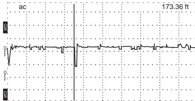
Figure 3-7: System 1 - Tap Quite Visible (128 avg, 50 ft/div, 35 dB)
