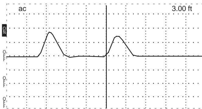
Figure 1-7: Vp Set at .66, Cursor on Rising Edge of Reflected Pulse (Set Correctly)
